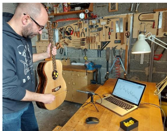
This is how we perform frequency response measurements in our workshop.
