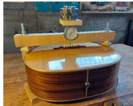
A dedicated jig with a micrometer and a weight is the setup necessary to measure the compliance of the soundboard, and then calculate the monopole mobility.
